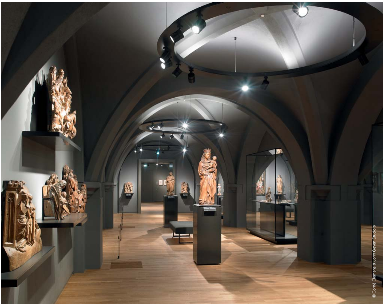
Top: Circular light rack from below, lighting effect on the left, technical Fortimo LED strip position on the right. Bottom: The lights are attached to specially designed slender black “racks” suspended from the ceilings.
